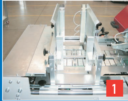
IN-FEED HOPPER: The book hopper can be manually fed or linked to a production line through a telescopic conveyor feeding from left, right or straight.
