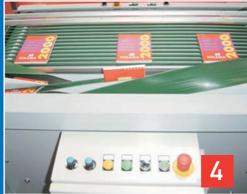
CONTROL BUTTONS: The control buttons are placed either on right and left side to easily operate the machine in the different configuration.
