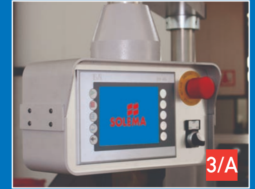
AUTOMATIC MAKEREADY: Optionally the machine can be endowed with DC motors for automatic size change of the hopper. Size change data are entered through the multi-line operating panel.
