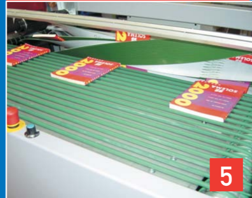
FLIPPING STATION: The Wendeband turning conveyor can be used to turn products upside-down for proper orientation.
